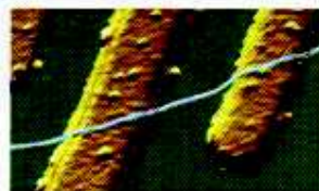
Nanowire (blue) on platinum electrodes (yellow) Magnification: x 120,000
